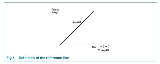
The angular range is set to  $\alpha_{max} = 180^{\circ}$  and the clamping voltages are programmed to  $V_{(CL)I} = 5 \ \% V_{DD}$  and  $V_{(CL)u} = 95 \ \% V_{DD}$  for a valid definition of errors.
